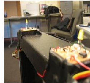
Figure 2: Occupancy Detector Circuit mounted on frame.
